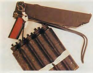
Designed for use against helicopters, parachute flares filled with wire-wrapped Flex-X can be fired singly by pull-cord or by means of this shoulder-held nine-tube launcher. The maximum effective range is 600 to 700 meters.
